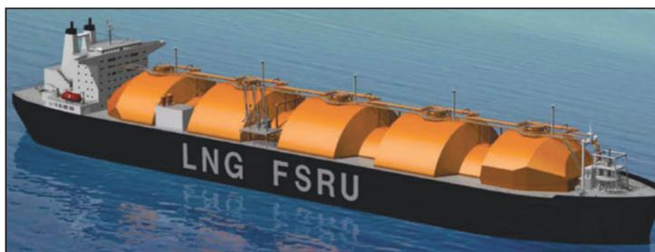
Looking to the future: a Golar Energy LNG concept for a floating storage and regasification unit, based on the conversion of an older LNG vessel.
