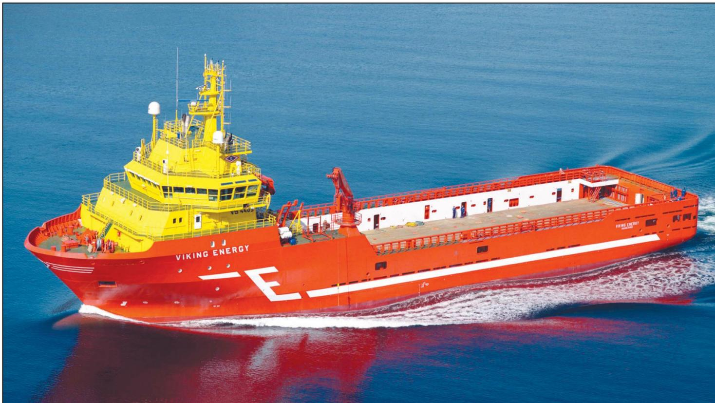
Eidesvik's Viking Energy: it is one of a number of dual-fuelled vessels that have influenced Harvey Gulf's decision to introduce fuel substitution. The vessel runs on either liquefied natural gas or diesel.
